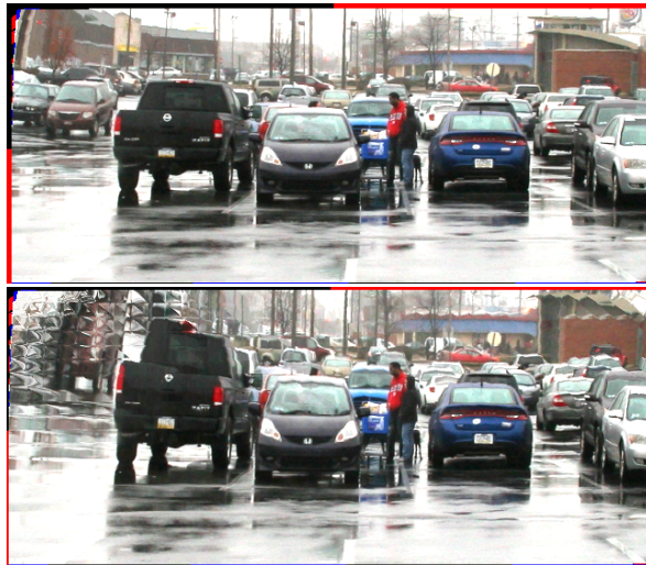
Fig. 10. Images of the test pattern (placed at different positions) via collimated bundle with r = 3 and no twist. We can see from the distortion in the lower image that the bundle is not perfectly collimated.
