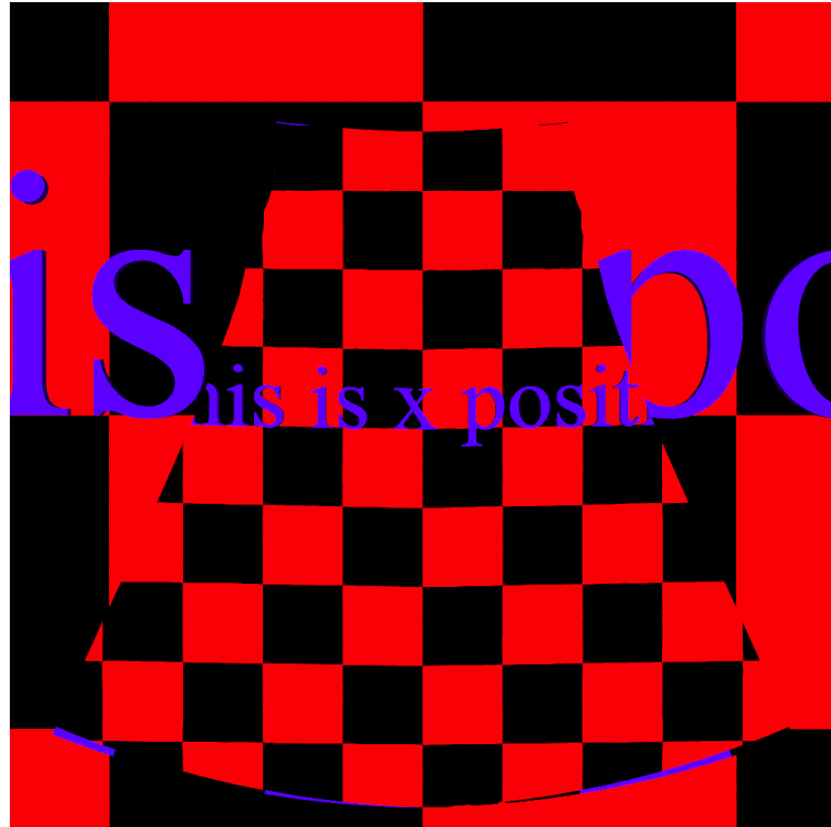
Fig. 11. A raytracing simulation of the mirror pair in Fig. 10.
