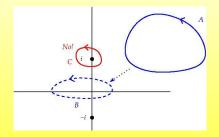
1. You have to deform the contour without crossing any singularities. In the picture, contour A can be deformed to B but not to C. It can't enclose the singularity i if it didn't already.
