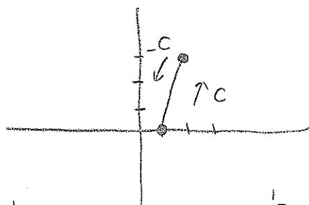
THEN  $\int_C P dx + Q dy = \int_0^1 P(dt) + Q(3dt) = \int_0^1 (P + 3Q) dt \quad \begin{pmatrix} x = t+1 & y = 3t \\ dx = dt & dy = 3dt \end{pmatrix}$
