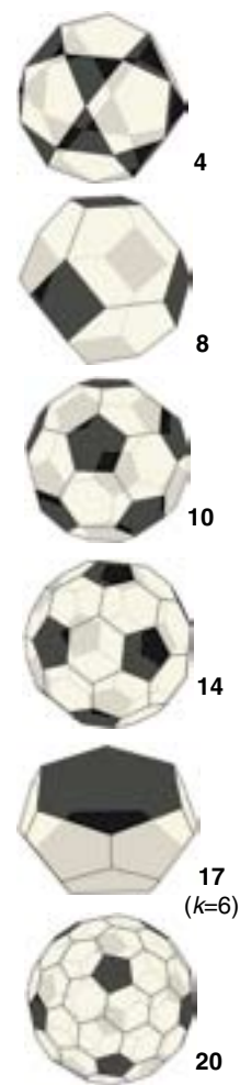
Figure 9. Generalized soccer balls fall into 20 types. In this table, k represents the number of sides in any black face; the product m \times n is the number of sides in any white face. Every side of a black face meets a white face. Every n th side of a white face meets a black face. The columns b and w represent the number of black and white faces in the simplest representative of each type. For the types with n=2 , every generalized soccer ball of that type is a branched covering of the simplest one. However, this is not true for other values of n . The minimal realization of type 8 is combinatorially the same as the 2006 World Cup ball shown in Figure 2, whereas type 10 is the standard soccer ball.
